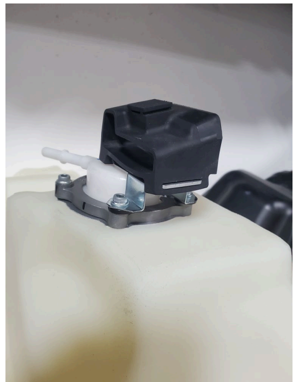
Fig. 3 ( IMS recommends running the larger zip-ty through the slotted holes on the black cover, and then underneath the seat hook style bracket to ensure the cover does not detach )
