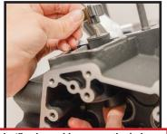
Use plastic knob to tighten down firmly (firmly pushing up on the bolt from below will help reduce effort needed). Repeat on other 3 lifter bores
