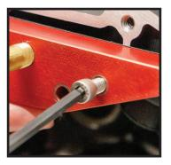
3. Slowly open regulator and record when the jet opens. 12-18psi is a typical range.
