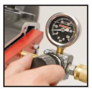
If the top end is removed, you can spray some oil onto jet to see when it opens. You may also intermittenly block the jet with a finger as you bring up the pressure, while watching for movement in the gauge needle. If the gauge needle raises when jet is blocked, the jet is opening. Be sure to inspect for any leaks around base of piston cooling jet.
