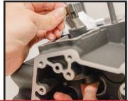
Use plastic knob to tighten down firmly (firmly pushing up on the bolt from below will help reduce effort needed). Repeat on other 3 lifter bores
