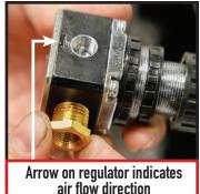
2. Apply Loctite 545 to other end of NPT stand off and install regulator with thread reducer.
