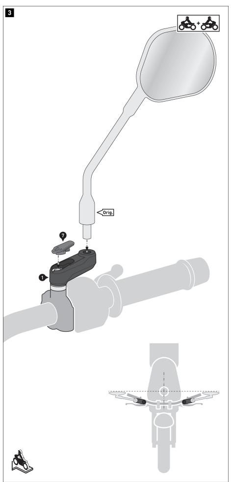
⚠ **NOTE:** Keep in mind the opposite thread directions of the original mirrors (Orig.): **Right side of vehicle:** Left-hand thread. **Left side of the vehicle:** Right-hand thread.
